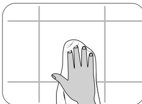
2. Clean the mounting place carefully with standard commercial cleaning agents and take care that the mounting place is completely free from dirt, dust and grease.
