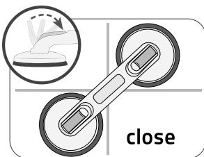
4. Press the grab handle with pressure at the mounting position on the wall and close the fixing lever. Hereby the vacuum arises.
