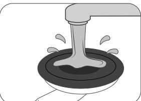
7. Possible residues of dirt, or similar on the suction cup can be removed with water and standard commercial soapy water. Do not use solvent-based, acidic or abrasive cleaning agents! After proper cleansing, the grab handle is ready for use again. Please respect steps 1. - 5.
