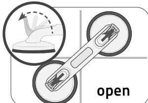
6. For disassembly open the fixing levers and take the grab handle away from the wall.
